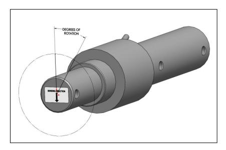
Underneath the cover is where all of the load cell circuitry is hidden away and protected from the elements. Without going into a lot of detail about how it all works, it's enough to say that the circuit is made of strain gages and other resistors wired into a Wheatstone bridge. The strain gages are positioned exactly on the top and bottom of the cell - that's how they are able to measure 100% of the load that is applied.
